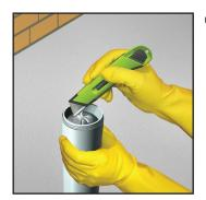
③ Cut the crimping clip using a knife or scissors.
